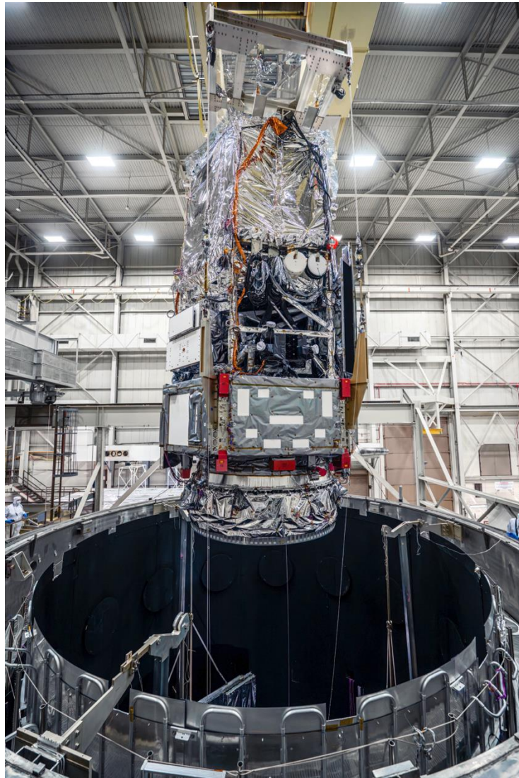
SCIPA lowering into SES chamber
